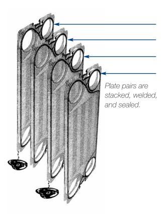
The feature that makes the Accu-Therm heat exchanger so useful — external leak protection — can provide double protection with its double-wall construction. Any hole in the plate surface allows the product to leak to the edge of the plate pair for immediate visual detection.
